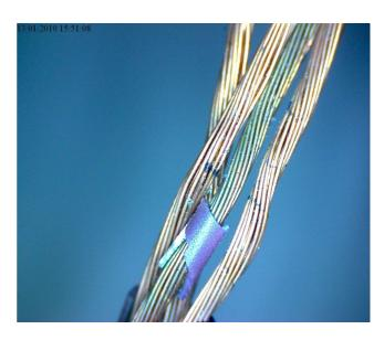
The plastic of the wire (probably PVC which withstands 70  $^{\circ}$  C) is cracked and the scales falls from the wire as soon as we move the cable.
