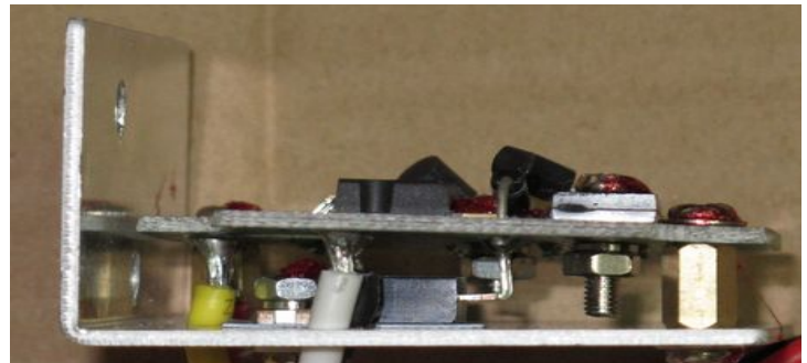
wires almost well soldered but not in the PCB holes (too small)
