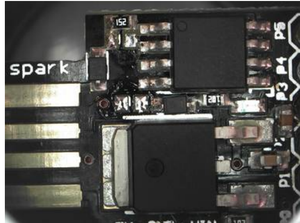
Without 68Ω resistors
